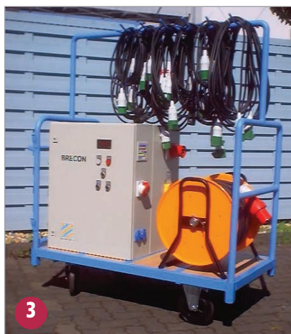
The end user contributes to details such as circumferential protective frame, single phase power outlet and power input on a cable drum
