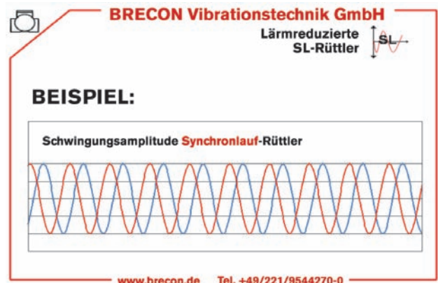
Fig. 5: the mechanical and electrical frequencies are only absolutely identical with the synchronous running vibrator; the exact rotary speed can therefore be read off from the frequency converter
