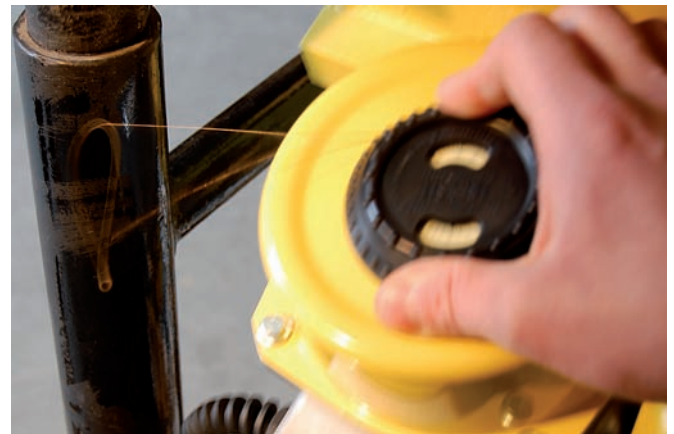
Fig. 4: The resonant oscillation indicates the momentary frequency
