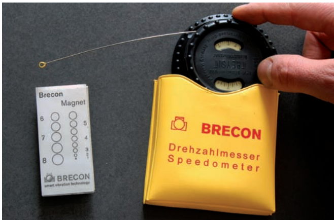
Fig. 3: The frequency measuring aid in a resting state
