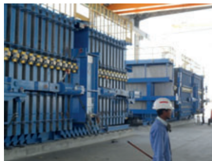
A total of 3 battery moulds with 2 x 10 chambers, 1 battery mould with 1 x 10 chambers, 231 Brecon high frequency external vibrator, 7 electrical distribution cabinets, 1 central frequency inverter cabinet and 1 Brecon radio control were installed.
