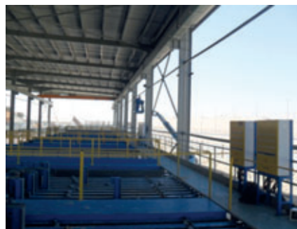
A total of 3 battery moulds with 2 x 10 chambers, 1 battery mould with 1 x 10 chambers, 231 Brecon high frequency external vibrator, 7 electrical distribution cabinets, 1 central frequency inverter cabinet and 1 Brecon radio control were installed.
