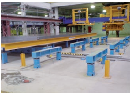
Fig. 9: Synchronous vibrator in the vibration station
