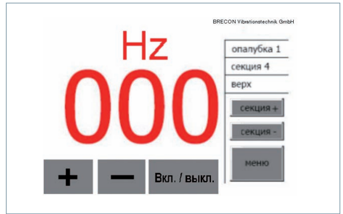
Fig. 7: Touch panel: The displayed vibration frequency can be adjusted at any time on the touch panel or via the radio transmitter. Adjacent to that, information on the form selection and vibrator verification.
