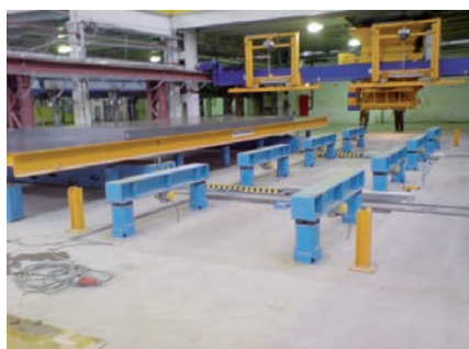
Fig. 9: Synchronous vibrator in the vibration station
