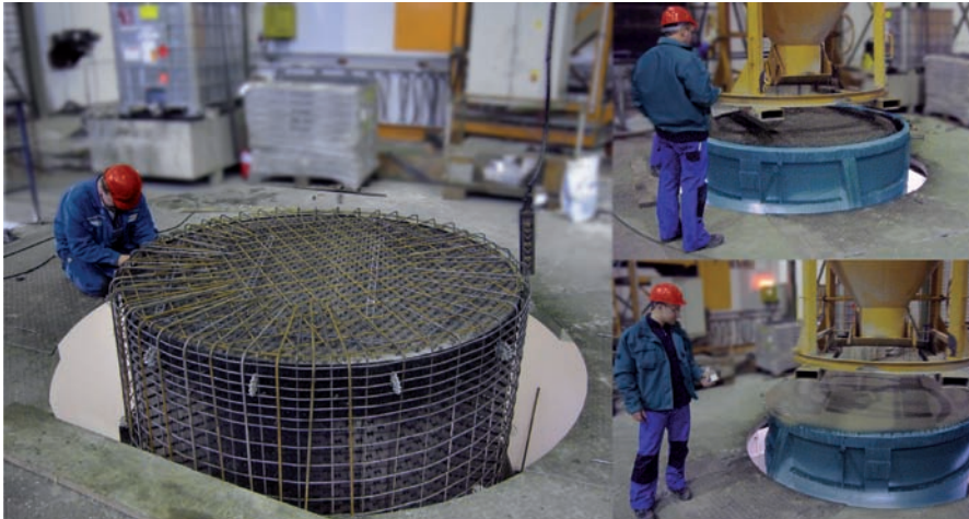
The two-step concrete compaction with Brecon 2in1 vibrators is advantageous at a high percentage of reinforcement.
